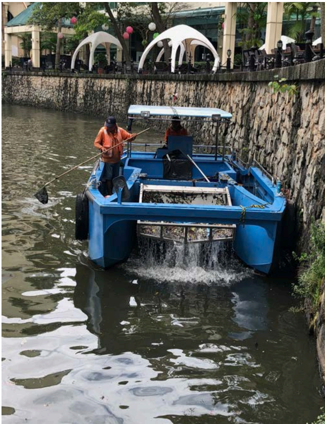
One of the trash removal boats that scour the river each day.
